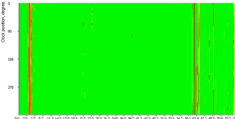
00 28 57 85 113 142 170 198 227 255 283 312 340 368 397 425 453 482 510 538 567 595 624 652 680 709 737 7 Length of pipeline, m The second shows how this information can be represented to show the density of anomalies (and therefore defects) in the axial plane and a more quantified representation of the degree of danger (ref y axis). Note that F (y axis) is an integral index of the degree
